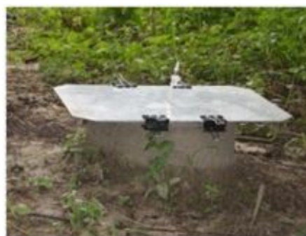
Figure 2: A static chamber measuring N 2 O and CH 4 fluxes on an oil palm plantation near Lahad Datu, Borneo. The chamber is sealed for 60 minutes. Air samples were withdrawn at intervals and sent to CEH, Edinburgh for analysis by gas chromatography.
