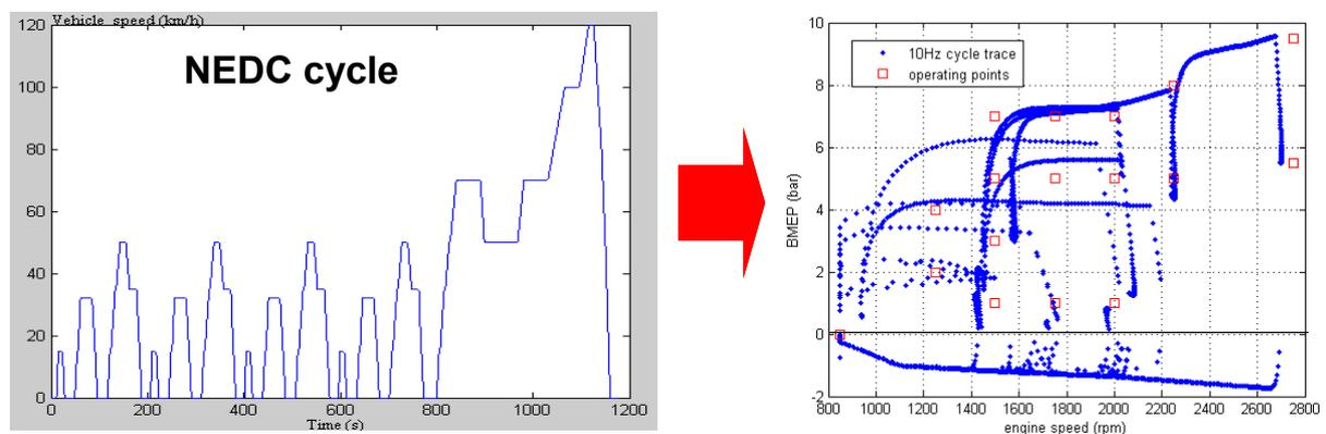
*Figure 1 Cycle simulation and selection of operating points*
