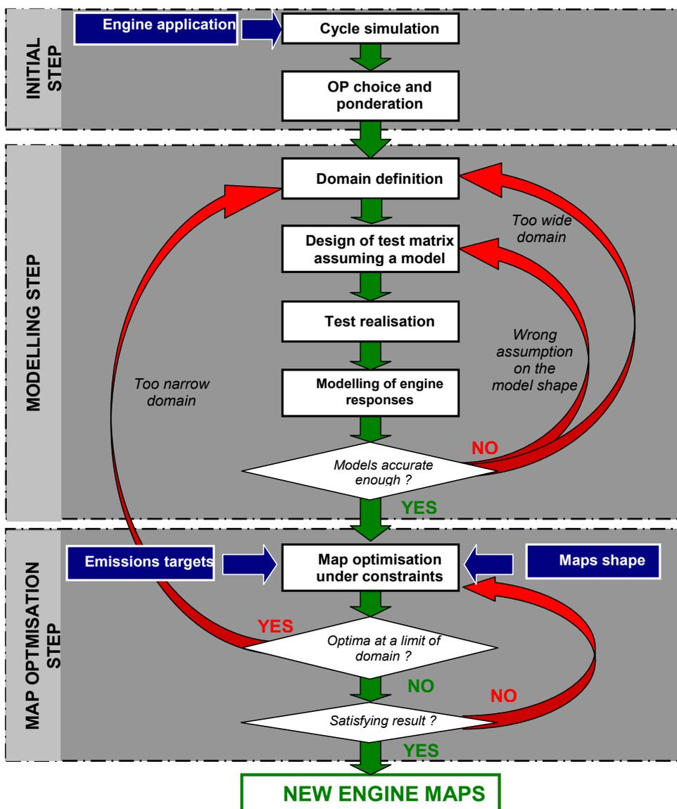
Figure 6 Flow chart of the mixed local method
