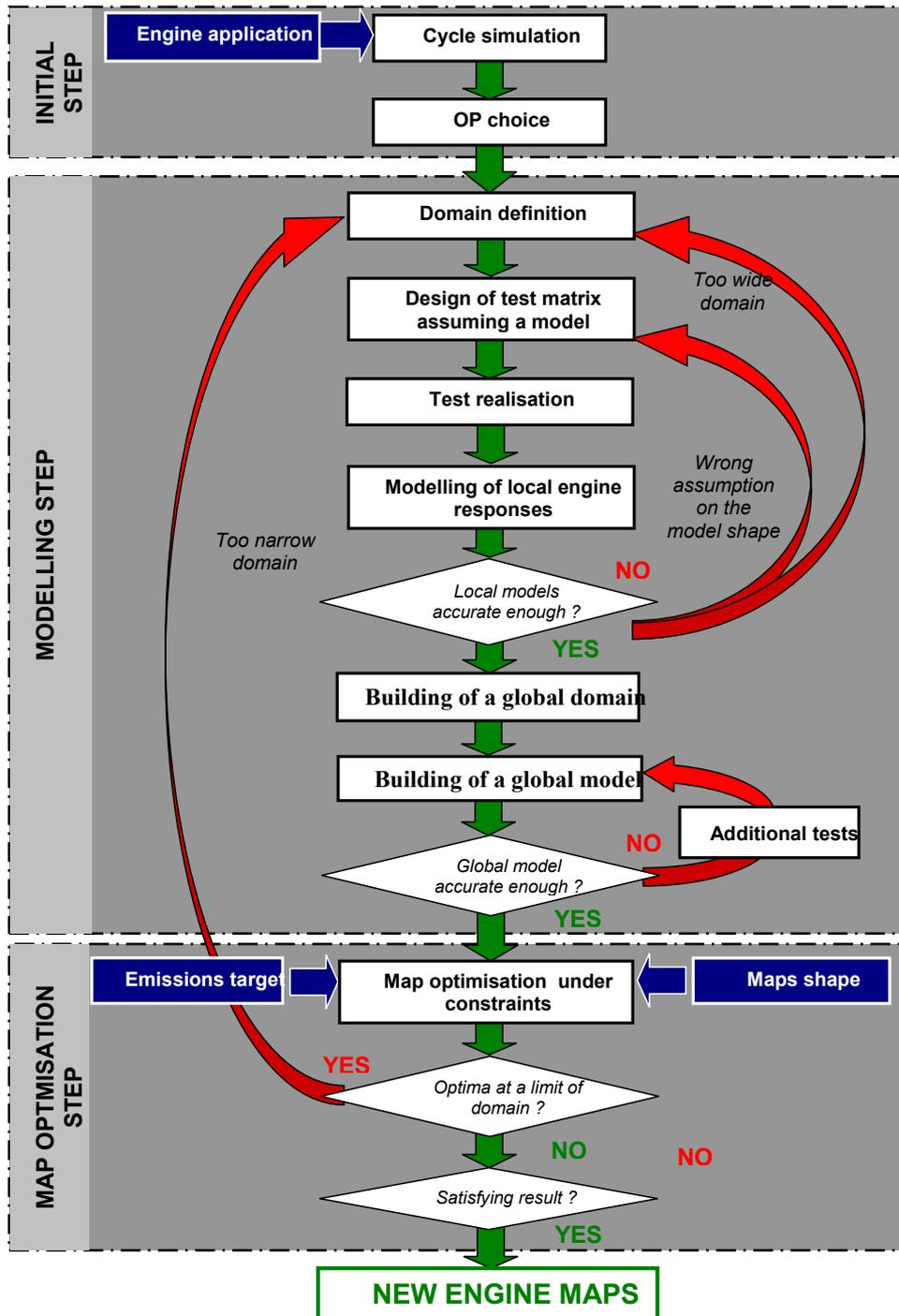
Figure 10 Flow chart of the indirect global method
