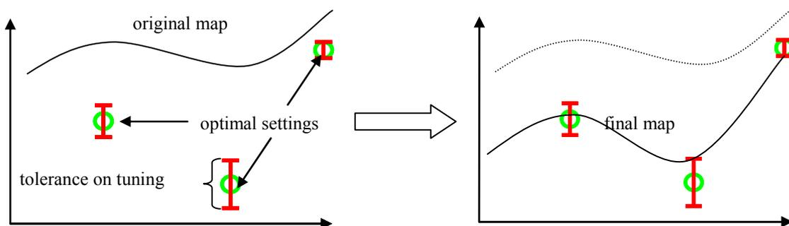
Figure 4 : Principle of IFP smoothing method
