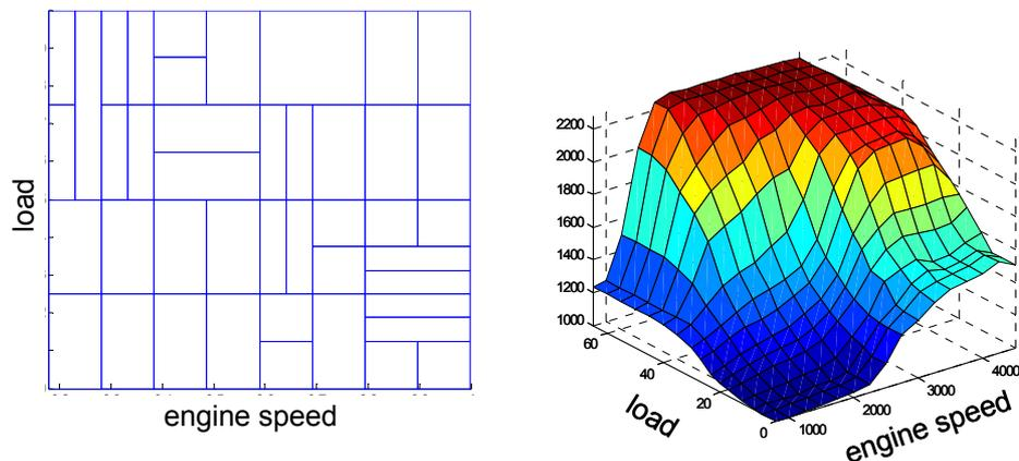
Figure 7 : Examples of LoLiMoT parameterization of engine map.
