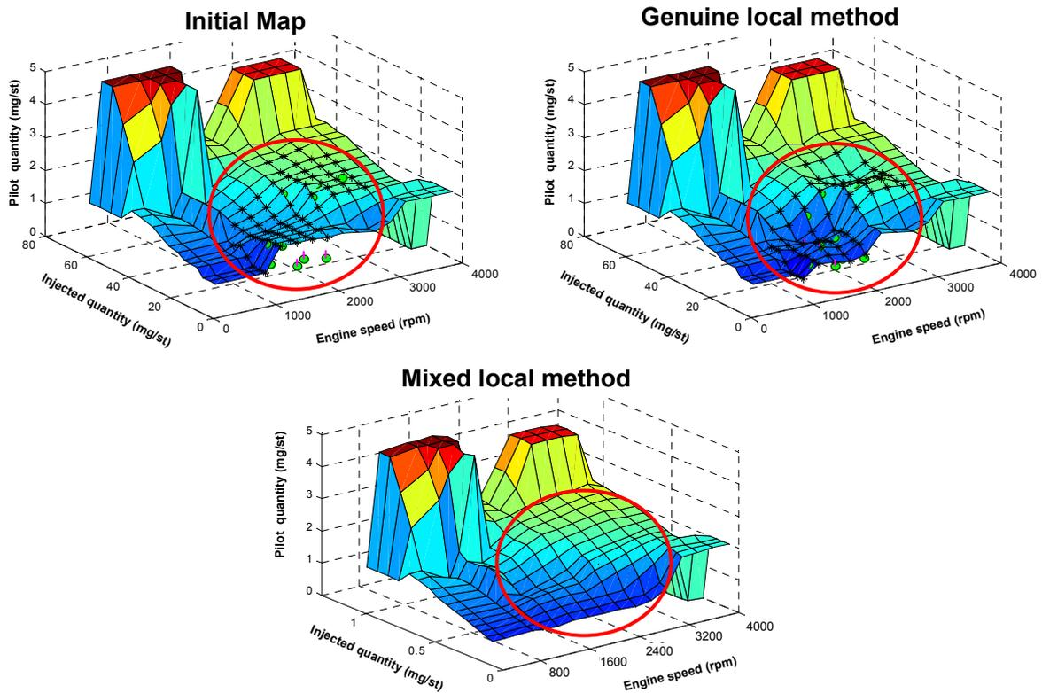
Figure 8 Comparison of pilot injection quantity maps
