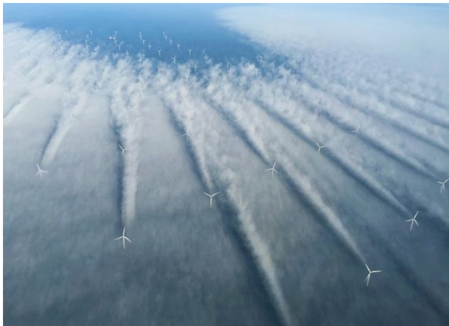
Figure 2.2: A naturally occurring visualization of the wake at the Horns Rev II wind farm off the West coast of Denmark [64, 63]
