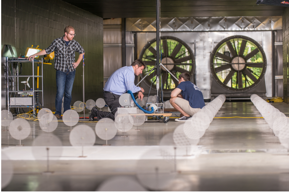
Figure 3.8: Photograph of the porous disk wind turbine array setup in the FPF. Looking downstream towards the low pressure plenum. Photo taken by Jeremy Gasowski
