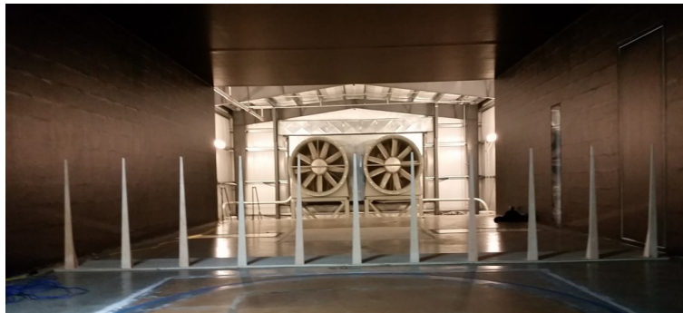
Figure 5.1: Irwin Spires placed at 62 m downstream of the inlet in the test section of the FPF
