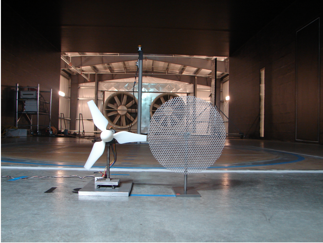
Figure 3.3: Side by side view of the porous disk and the rotating model turbine pictured in the rear of the FPF test section (61 m downstream of the inlet) looking downstream. Both models have diameter D = 0.25 m and hub height of 0.75 times D .
