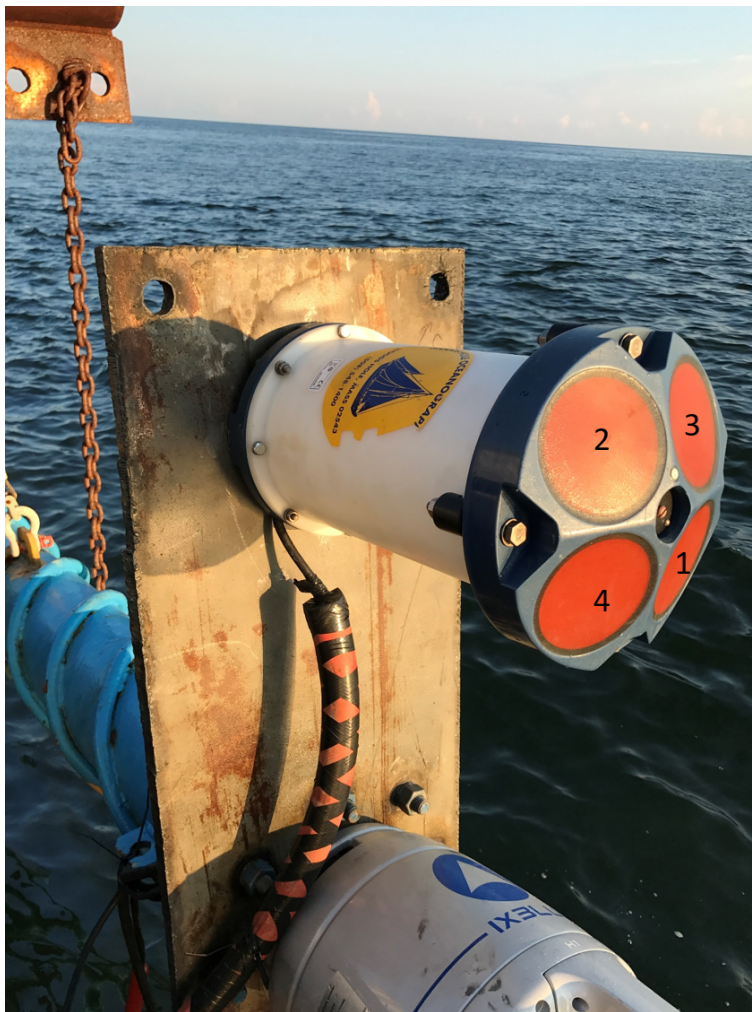
Figure 4.5: The orientation of the beams of the ADCP. The ADCP is pointing towards the bow of the vessel and is on the port side of the vessel in this image. The beams are labeled 1-4, with beam 3 the "forward" beam in beam coordinates.
