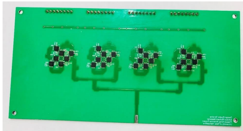
Figure 96: Fabricated Phase Shifters – phase shifter side.
