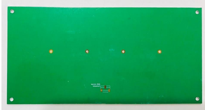
Figure 95: Fabricated antenna – ground plane side.
