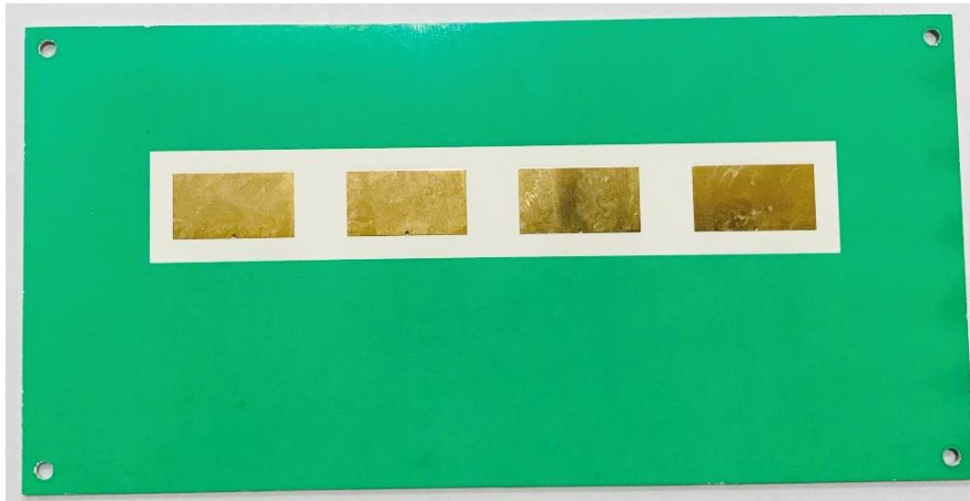
Figure 94: Fabricated antenna – array side.
