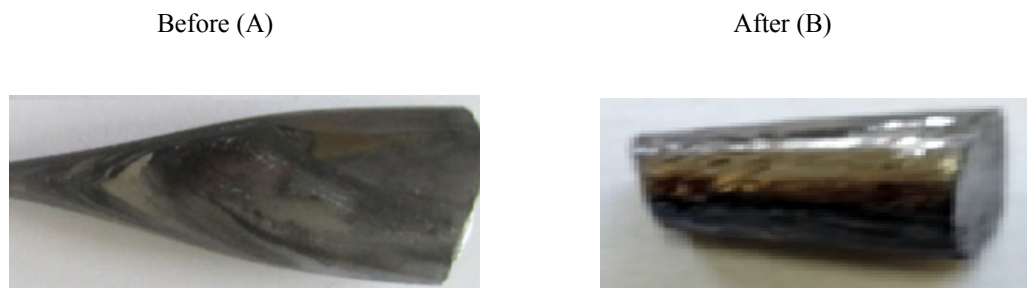
Figure 3. Pictures of the BiI 3 crystals without (A) and after three purifications (B)
