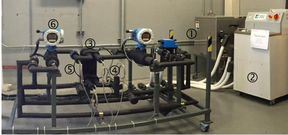
Fig. 4. Virtual borehole test bench (numbers correspond to instruments described in Table 1).
