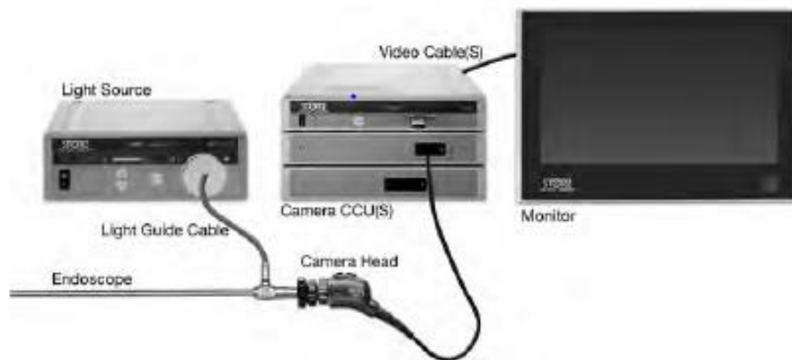
Figure 3 Basic endoscopic imaging chain, (2014 Photo Courtesy of Karl STORZ GmbH & Co.KG)
