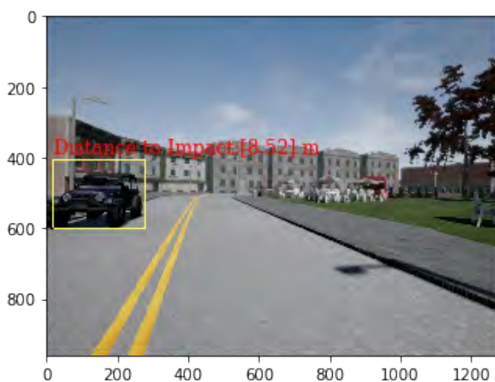
FIGURE 5.34: A showcase of calculating the distance until impact with the use of 3D image representation
