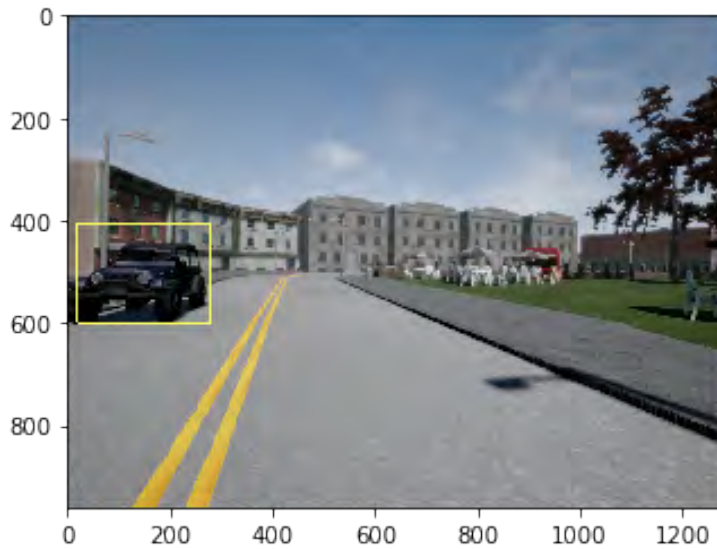
FIGURE 5.33: The result of filtering out object detection's unreliable results with the use of semantic segmentation
