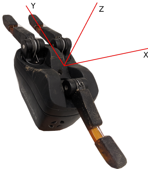
Figure 4.1: Figure showing the orientation of the reference frame centered on the palm of the ReFlex SF. The location of the origin is flush with the closest plane that can be placed on the gripper’s pads, and not with the center screw ( 1cm under the plane).
