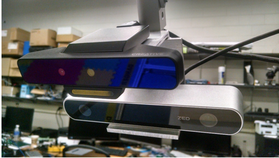
Figure 3.4: Early version of the mounting mechanism for the RGB-D cameras. Above: SR300, which after some tests we found would be better placed closer to the workspace. Below: ZED camera.
