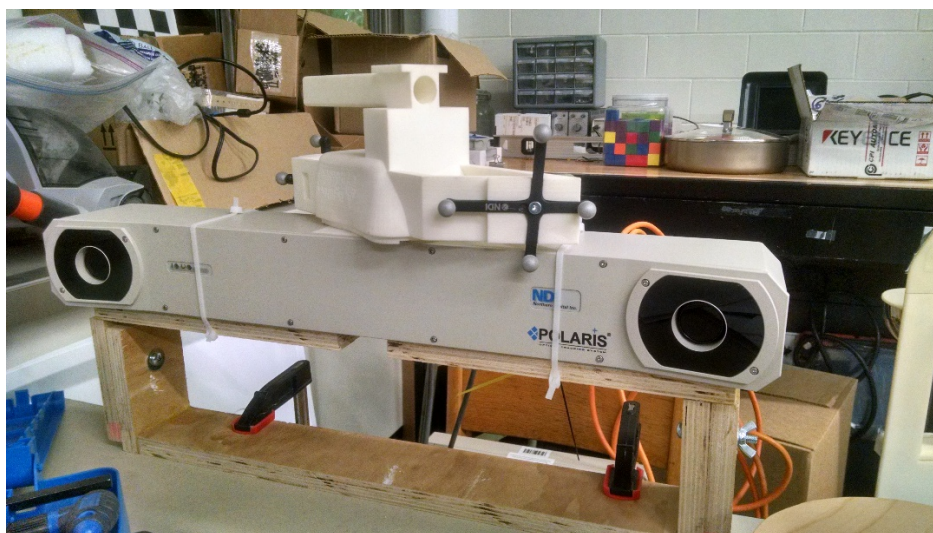
Figure 3.3: NDI Polaris and 3D printed gripper shell with IR tracker. The Polaris has two cameras placed at either end of plastic shell. Around each camera there are a series of IR emitters that are used to illuminate the IR trackers.
