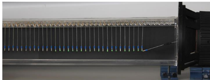
Figure 1.11: An array of pendulum magnets driven by a dynamic subwoofer speaker [16].
