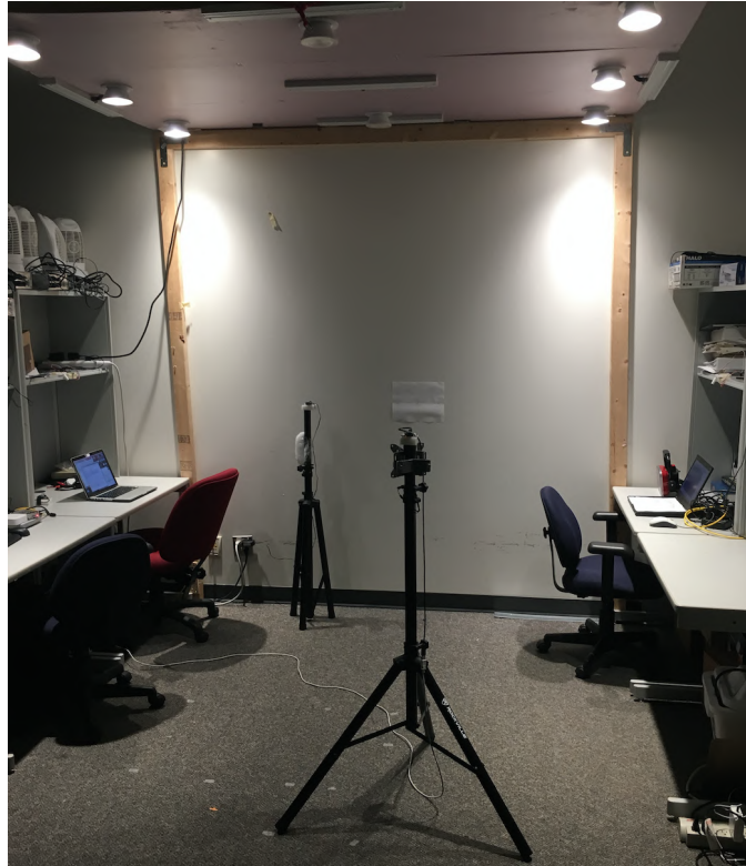
Figure 4.5: Experimental setup for evaluating the integration of portable sensing modules into the smart lighting system. Two portable sensing modules are mounted on the top of tripods.
