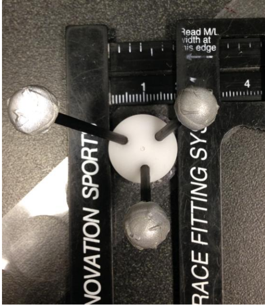
Figure 2.3 Custom made clusters of spherical markers used in the multi-segment foot model.
