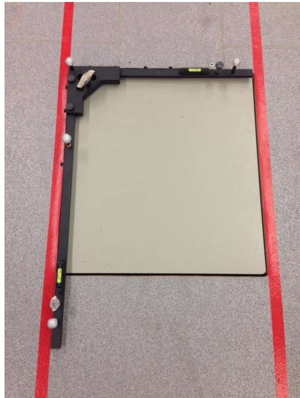
Figure 3.4 L-shaped calibration frame (seed frame) creating the axes of the lab. The four fixed markers help create a lab frame of reference.
