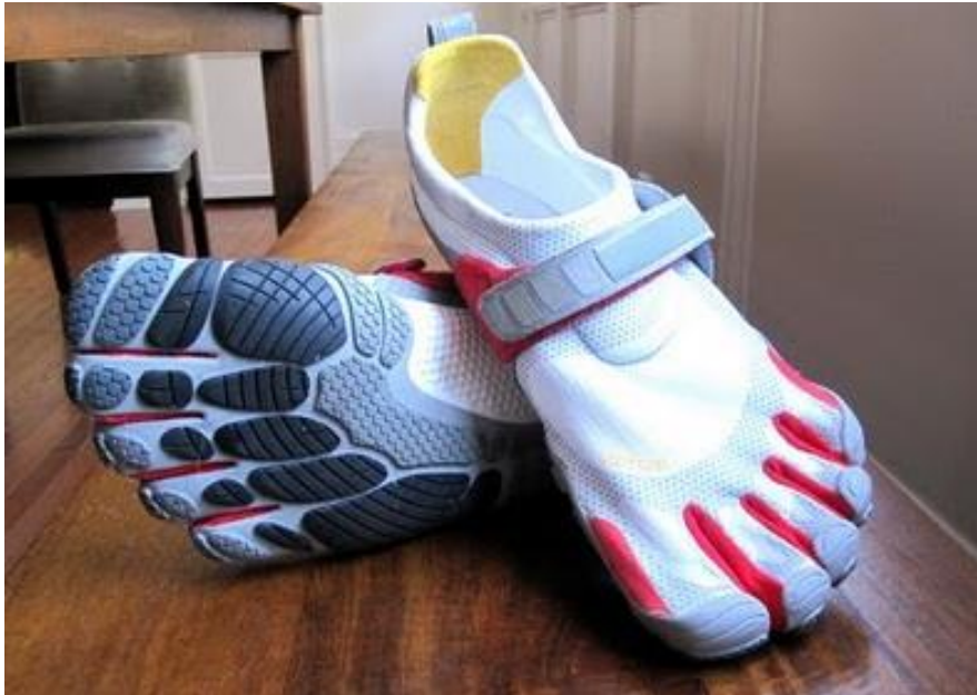
Figure 3.8 Vibram Five Fingers Bikila without holes for the multi segment foot model. Reflective patterns on the shoes were covered with athletic tape as to avoid interference with infrared lighting and marker recognition.
