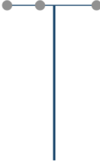
Figure 3.5 Calibration wand fitted with three fixed reflective markers used to calibrate the data collection area.
