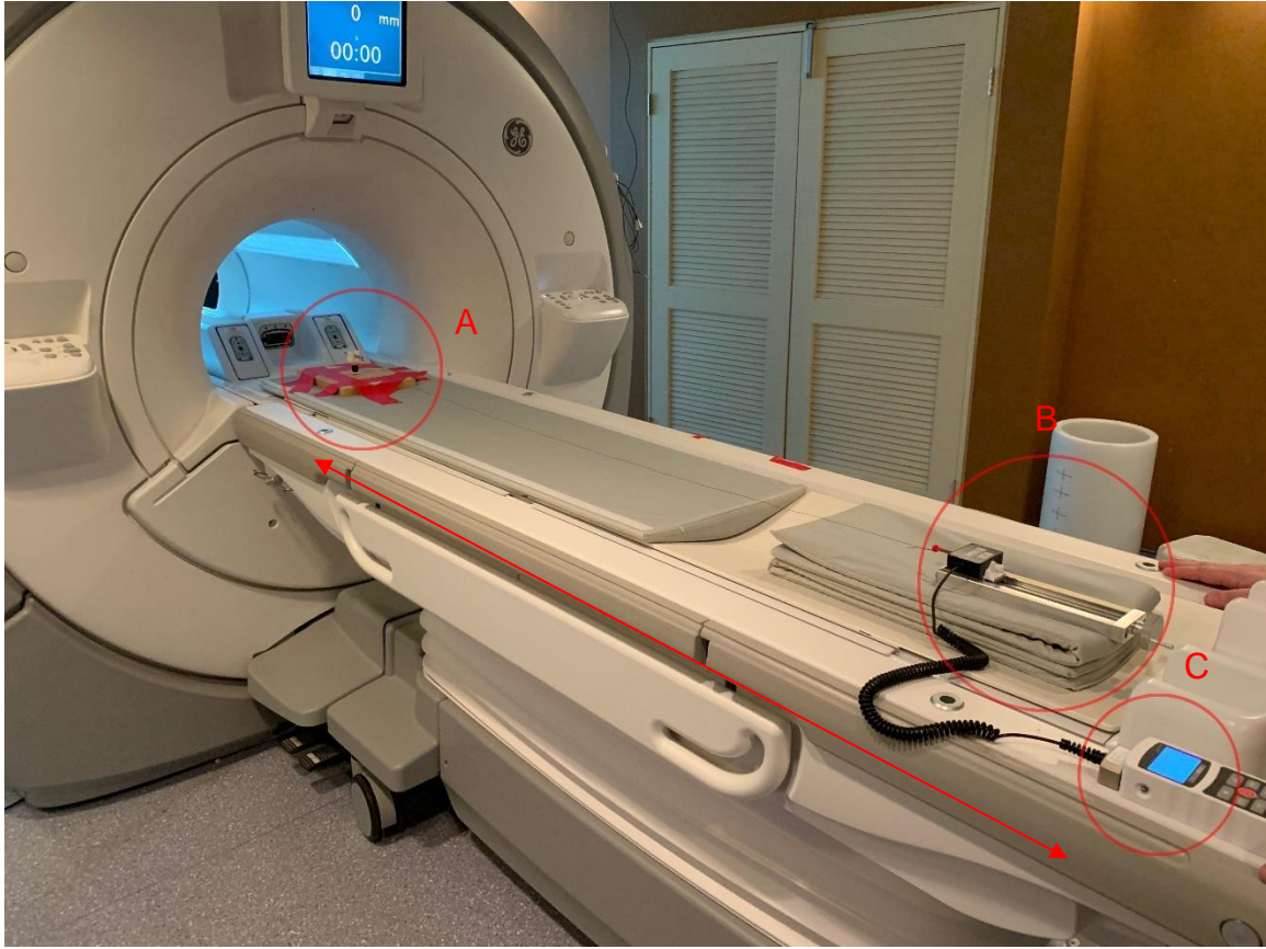
Figure 2-9: The apparatus holding the test cylinders (A) from figure 2-8 is fixed to the patient table of an MR scanner with tape. The linear displacement mechanism holding the force sensor (B) from figure 2-6 is positioned at a distance such that all equipment still functions accurately. The patient table is moved into the MR scanner to position apparatus (A). There is a thread extended from (B) to (A). As the force sensor moves away from the scanner, the device is rotated and the tension in the string is recorded with device (C). Device (C) is the digital meter displaying the force reading and zeros the force sensor.
