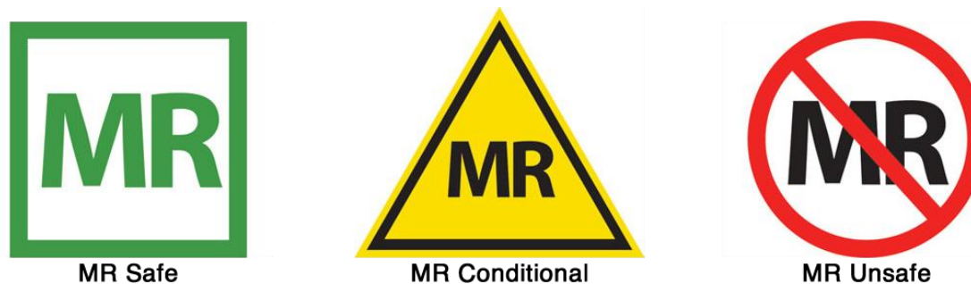
Figure 1.4-1: Symbols proposed by ASTM International in ASTM F2503-13 for MR Safe, MR Conditional and MR Unsafe [26]. Reprinted with permission from ASTM International, reference 26.
