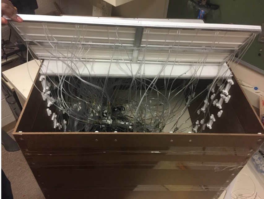
Figure 13. Pressure tap tube connections
