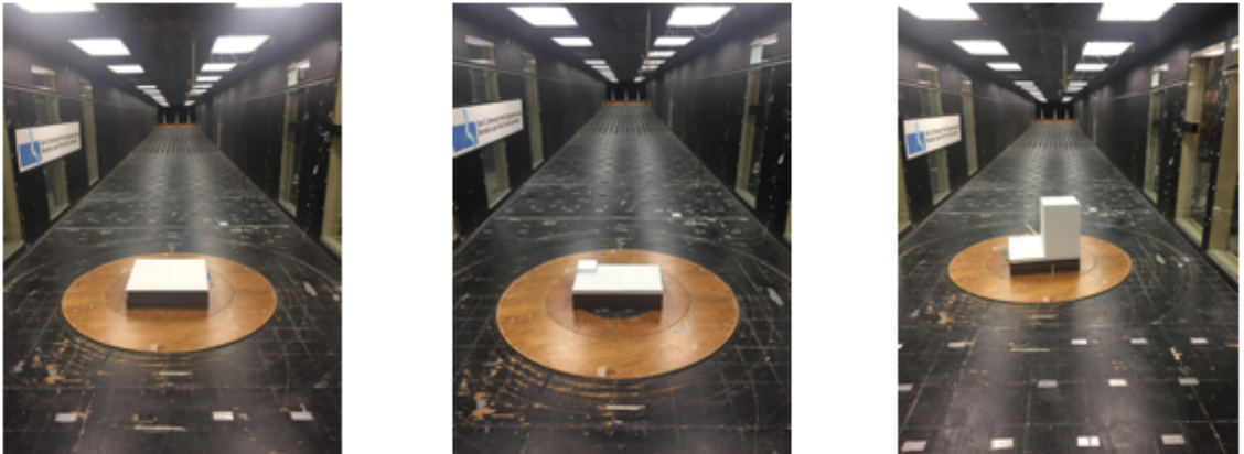
Figure 11. Small obstruction attachment at center of building roo
