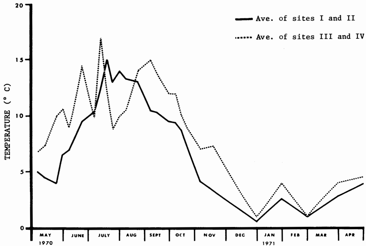
Fig. 7. A comparison of water temperature above and below the reservoir.
