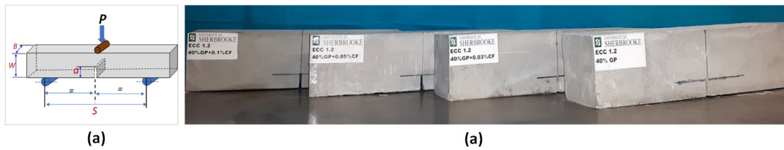
Fig. 6. Fracture toughness test: (a) Test set-up illustrating the variables used in Eq. (12), and (b) Test samples
