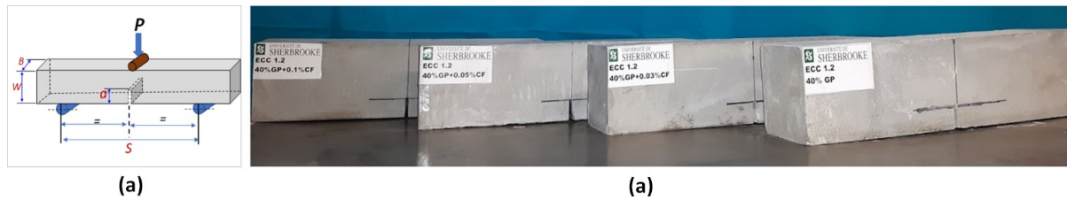
Fig. 6. Fracture toughness test: (a) Test set-up illustrating the variables used in Eq. (6), and (b) Test samples
