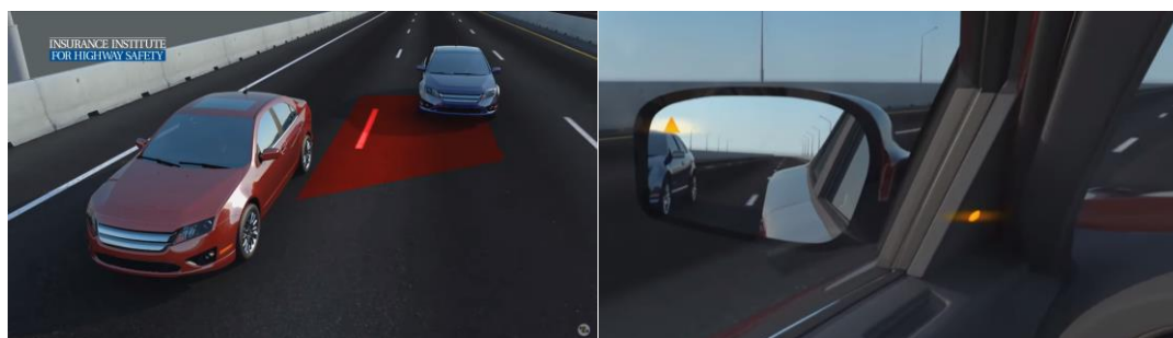
Figura 38. Blind Spot Detection IIHS (47).
