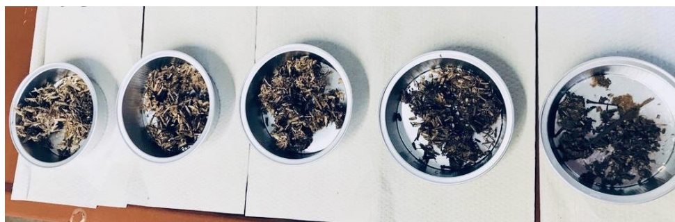
Figure 16: Photograph of standards solid samples for different residence times: 5 mins (left); 10 mins (middle-left); 20 mins (middle); 30 mins (middle-right); 50 mins (right)
