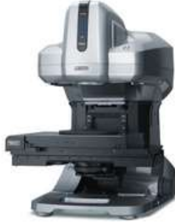
Figure 30 – Wide-Area 3D Measurement System VR-300 from Keyence.
