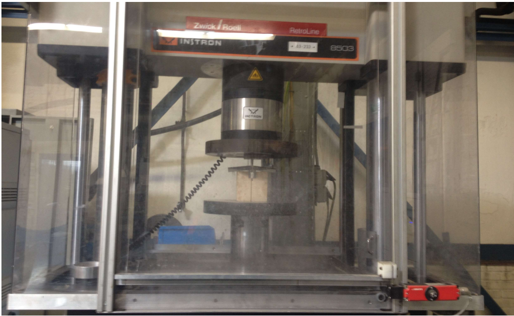
Figure 28 – Configuration of the wedge splitting test.
