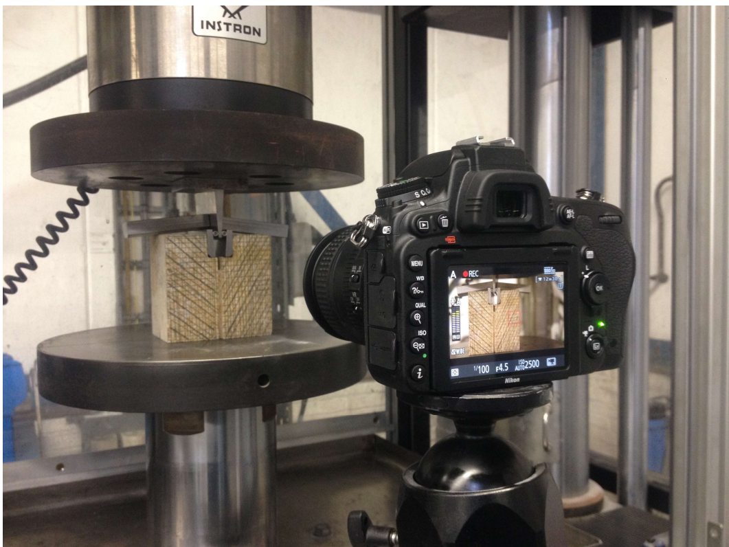
Figure 29 – Configuration of the wedge splitting test with DIC.
