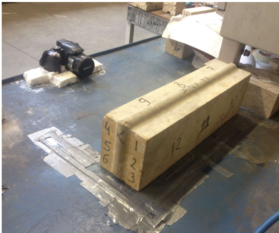
Figure 24 – Set up used throughout the cycles to capture the photos or DIC.
