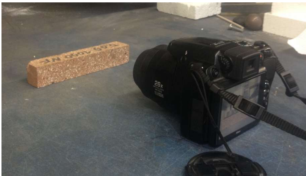
Figure 23 – Set up used to capture the photos for Digital Image Correlation.
