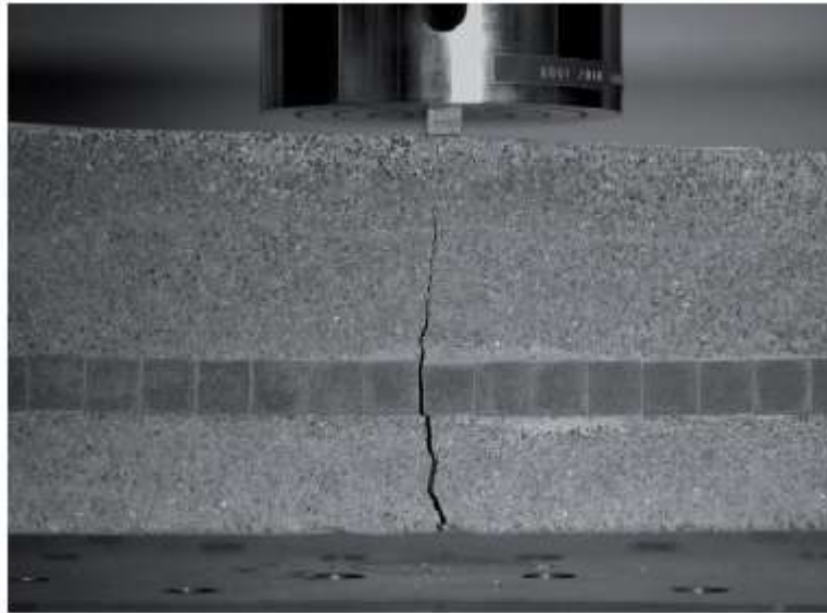
Figure 10 – Concrete step after being subjected to load test, showing one large crack but no other visible cracks [35].
