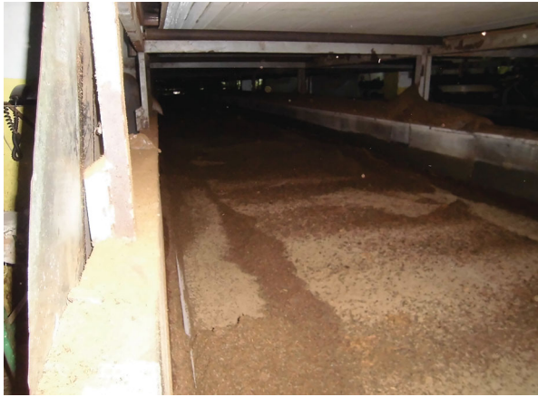
Figure 6. A fermentation band without curled tea in its entrance during the fermentation process.
