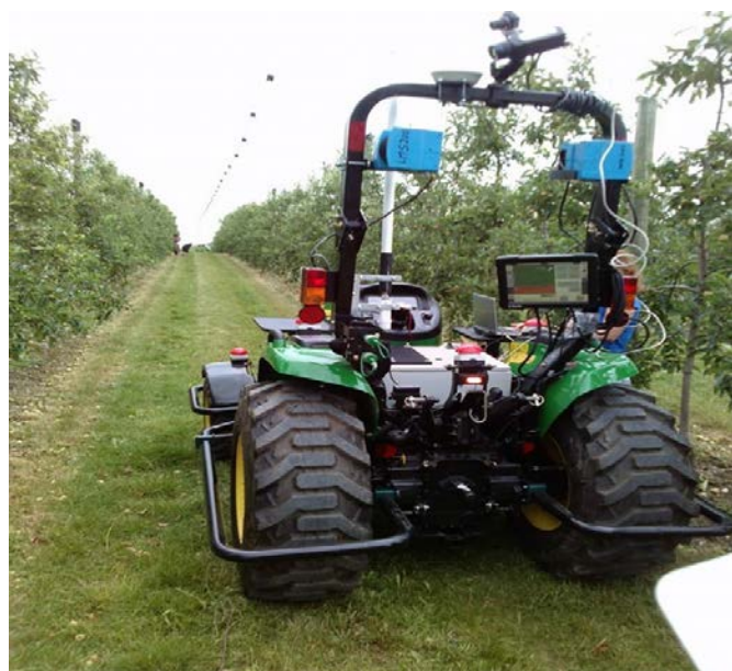
Figure 2. Sensors mounted on robotic platform during field data collection (Source: USERPA project portal)
