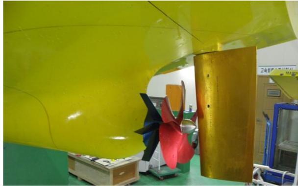
**Fig. 15** Experimental setup for the self-propulsion test
