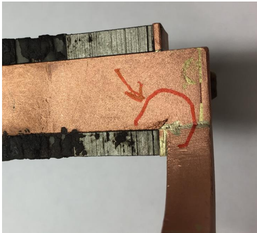
Fig. 3: Crack at the workpiece-facing corner
