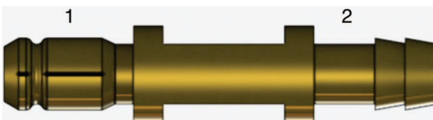
Figure 3: Connector to clamp samples into the test bench. Ending 1 is permanently connected to the tube networks. Vascular grafts are fixed on ending 2.
