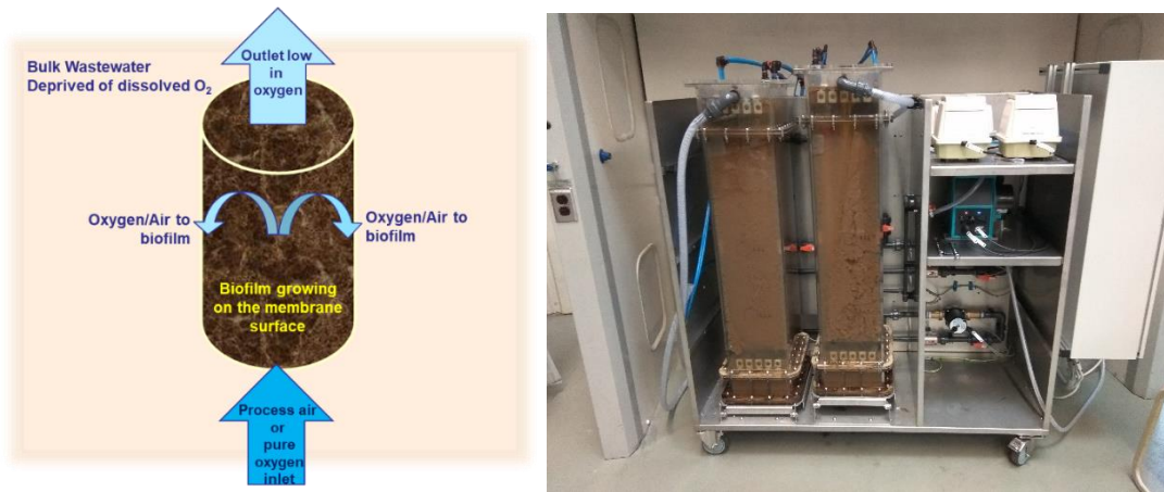
Figure 1 OxyMem MABR twin pilot at Dow, Terneuzen - main concept (left) and after inoculation (right)
