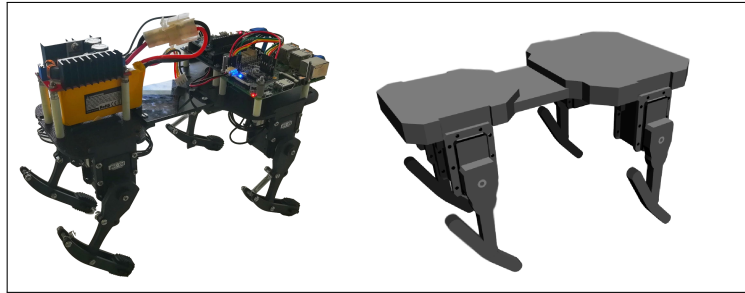
Fig. 2. Tigrillo physical robot (left) and model (right).
