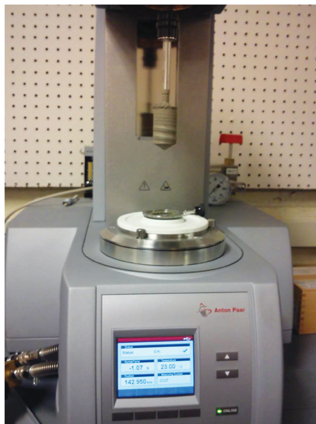
Fig. 1—MCR rheometer; equipped with sandblasted coaxial cylinders.
