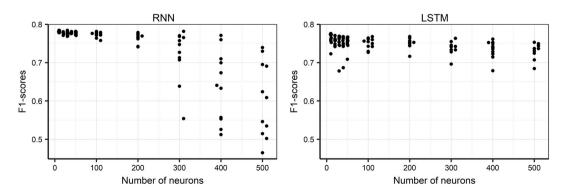
FIGURE 6 F1-score (measure of model performance) as a function of model architecture (number of neurons, indicating complexity) for recurrent neural network (RNN) and long short-term memory (LSTM) RNN alternative prediction models. A high F1-score indicates a better performing model
