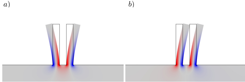
Figure 3.3: Mechanical supermodes of the cantilever pair. The colors signify the volumetric strain.
