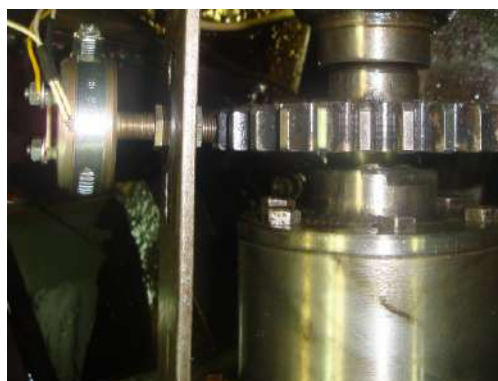
Fig. 6. Inductive speed sensor mounted on the shaft of the powder brake mechanism
