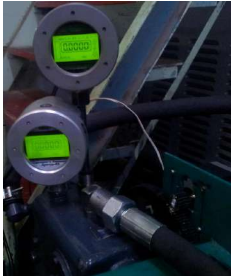
Fig. 5. "Arktur-03" overpressure sensors
