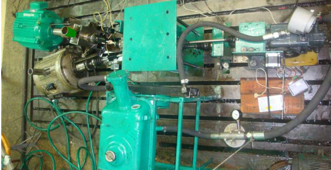
Fig. 3. General view of the stand of HSMT with an output differential
