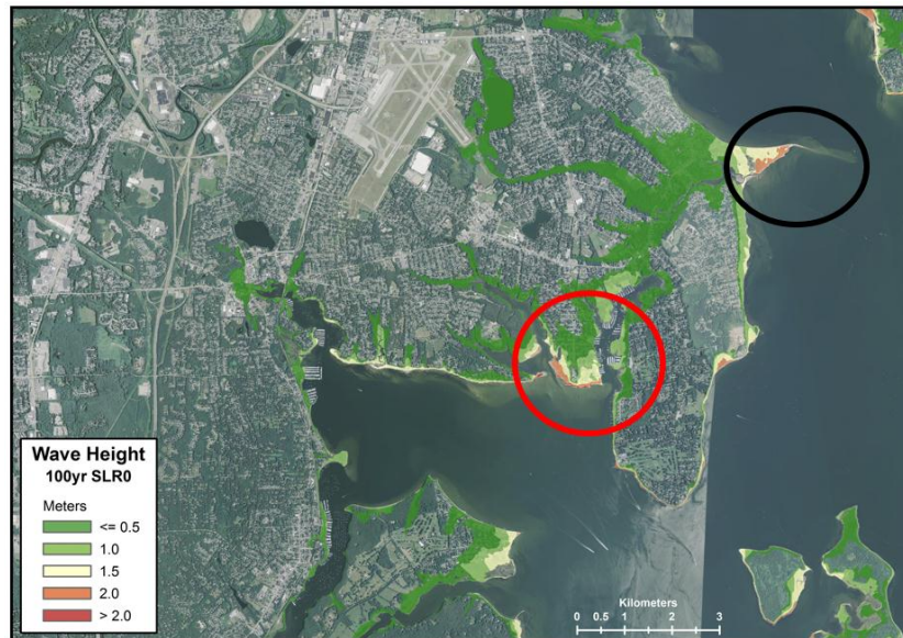
Figure 12. Controlling wave height (m) for Warwick, RI, 100-year event. Areas with substantially larger wave heights are shown; red circle for Oakland Beach and black circle for Conimicut Point.
