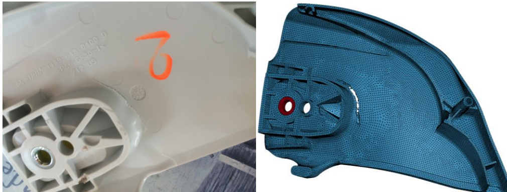
Figure 14 – Comparison of results and simulation of the custom drop weight test
