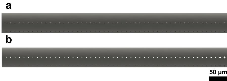
**Figure 15:** (a) CAD rendering of the unoptimized tubule design with consistent pore radii. (b) CAD rendering of the optimized tubule design with variable pore radii.
