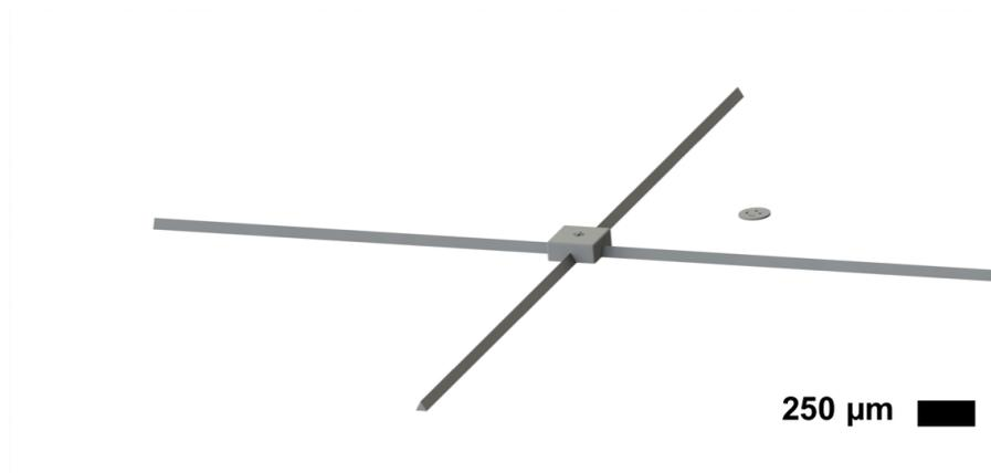
**Figure 32:** CAD rendering of the mold used to fabricate microfluidic devices with triangular channels. The width of the central chamber is 250  $\mu\text{m}$ .
