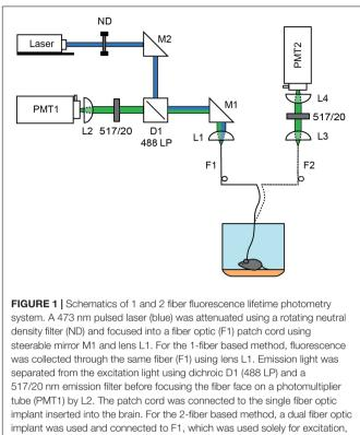
and to a second fiber optic (F2) patch cord used to collect fluorescence. The F2 fiber face was imaged onto a PMT (PMT2) using lens L3 and L4 which were separated by a 517/20 nm emission filter. In each case, the PMT was connected to a time correlated single photon counting board.
