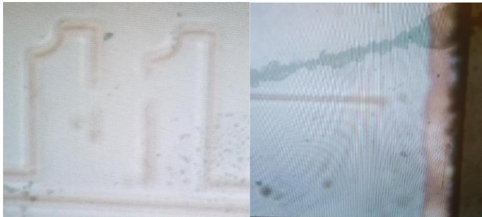
Figure 8: At left, pixel channels are under-etched, possibly a result of underexposing the pattern. At right, an etch line did not reach the edge of the device. ITO removed (pink) from edge did not reach the regional boundary.
