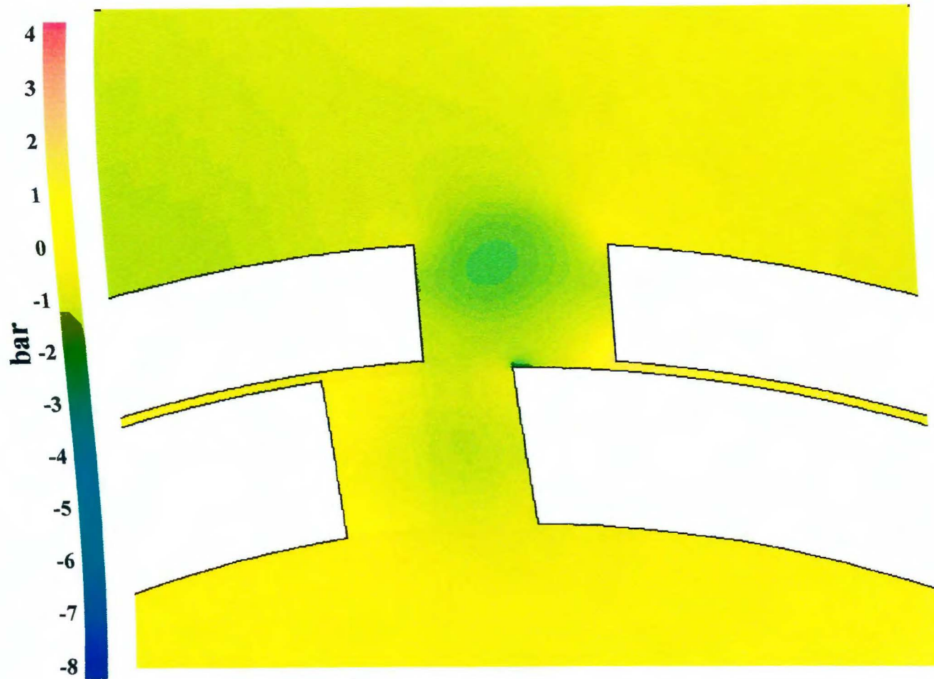
Figure 5-35. Angularly resolved mean static pressure near slot 1 at time step 6,416 (0.6436 seconds). Simulation 5.
