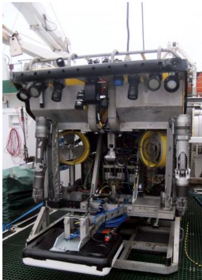
Fig. 4 The Holland 1 ROV. Note lights, cameras and manipulator arms.
