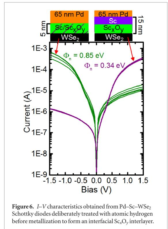
**Figure 6.**  $I$ - $V$  characteristics obtained from Pd-Sc-WSe<sub>2</sub> Schottky diodes deliberately treated with atomic hydrogen before metallization to form an interfacial  $\text{Sc}_x\text{O}_y$  interlayer.
