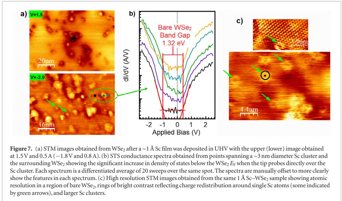
high resistance tunneling barrier and therefore fewer occupied LDOS. Sc oxidation occurs in UHV and therefore could contribute to the suppressed LDOS around Sc when ‘filled’ states are probed.
