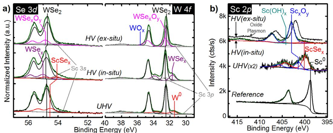
**Figure 1.** (a) Se 3d, W 4f, and (b) Sc 2p core level spectra obtained *in situ* after Sc deposition in UHV and HV on bulk WSe<sub>2</sub> (base pressure  $< 2 \times 10^{-9}$  mbar in each case, see Methods for details on the deposition in HV). Significant reactions occur between Sc, WSe<sub>2</sub>, and background gases in the chamber, which completely convert Sc and ScSe<sub>x</sub> to Sc<sub>x</sub>O<sub>y</sub> when the deposition is performed in HV.
