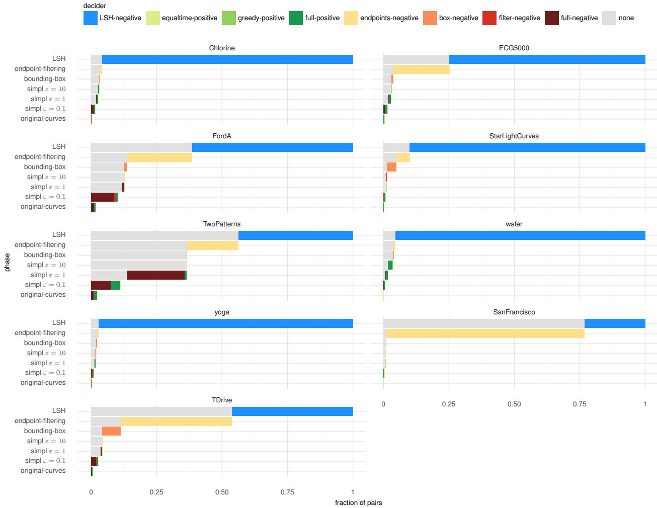
Figure 7: Breakdown of the effect of the various heuristics used to decide whether a pair is a positive match or not. The hue of the colors increases with the cost of the heuristic, so full-negative is more expensive to compute than endpoints-negative .
