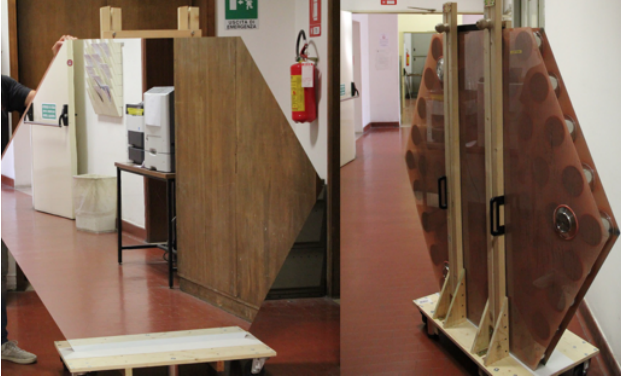
Figure 4: Prototype mirrors produced with the thin glass replica method. The mirror has a diameter from edge to edge of 1.5 m. The mirrors for Trinity will be square with a length of 0.5 m to 1 m.
