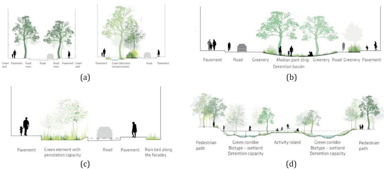
Figure 4: Typological road sections of Cloudburst solutions for the city of Copenhagen: stormwater roads (a); detention roads (b); detention areas (c); green roads (d). SLA Landskabsarkitekter. Source: The Municipality of Copenhagen
