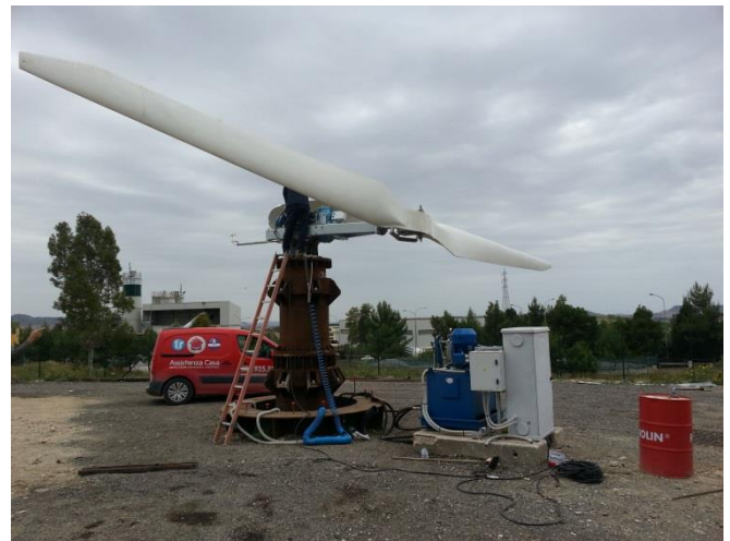
Fig. 1 PERIMA prototype with telescoping tower in its lowered position
