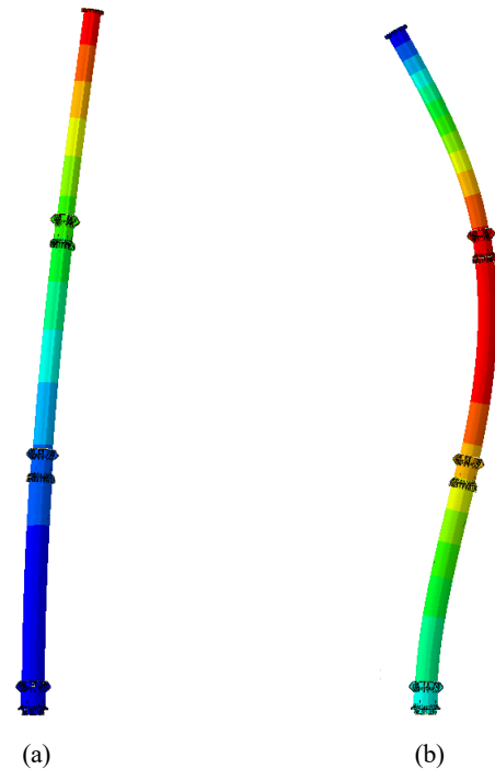
Fig. 15 Wind tower mode shapes: a) first mode (frequency 0.61 Hz), b) second mode (frequency 3.483 Hz).
