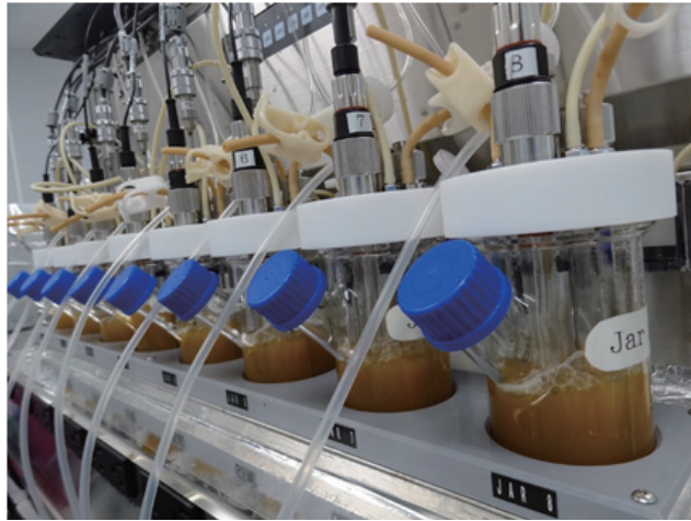
Supplementary Fig. 1. Kobe University’s Human Intestinal Microbiota Model is a single-batch fermentation system composed of eight parallel and independent anaerobic culturing vessels
