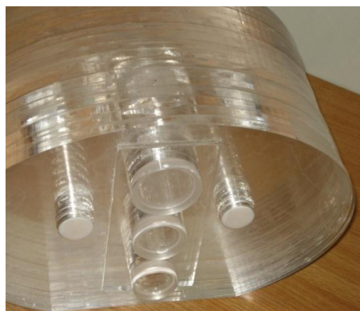
Figure 1: A View of Constructed Pelvic Phantom
