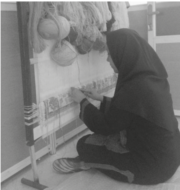
Photo 1. Workstation A: a low height vertical loom and a weaver sitting on the floor in a cross-legged position, without any backrest
