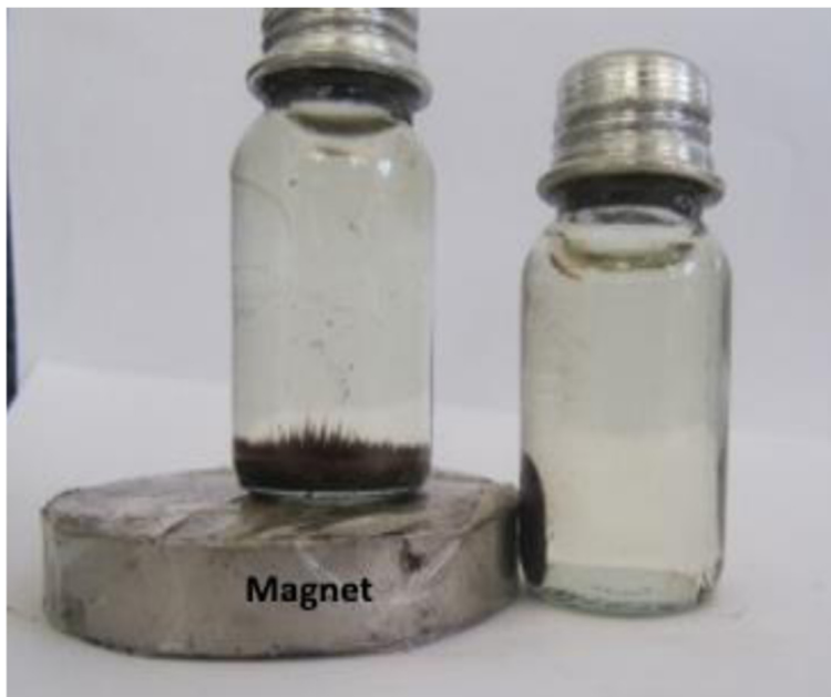
Fig. 3 Demonstration of magnetic separation at 30 s
