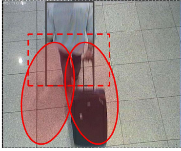
Figure 2. Spatial context for a person and a trolley: the 2D detection of the person (solid gray line) allows to derive a 2D image area in which to search for a trolley (red dashed line). However, the 2D context does not take into account 3D perspective changes (e.g. a large camera tilt as shown here). In contrast, the projected 3D context (see figure 6) models the search area more accurately (red solid line).
