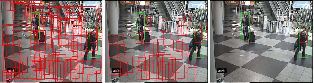
Figure 7. Filtered detections after each processing step (cf. figure 3). Initial 2D detections (left) of humans (green) and backpacks (red) show the difficulty of detecting inconspicuous objects. After 3D auto-calibration, detections which are inconsistent with scene scale and geometry can be removed (center), but different luggage types still cannot be differentiated reliably. When applying the 3D context model centered around the human detections, the precision of the backpack detector is significantly improved (right).
