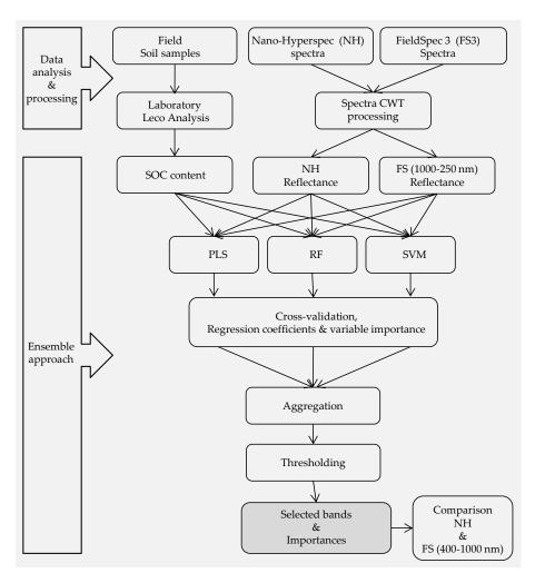
**Figure 3.** Flowchart of the methodology (i.e., analyses, processing steps, and the modeling) used in this study. A detailed description of the ensemble multimethod is provided in Reference [18]. PLS: Partial least squares; RF: Random forest; SOC: Soil organic carbon; SVM: Support vector machine.
