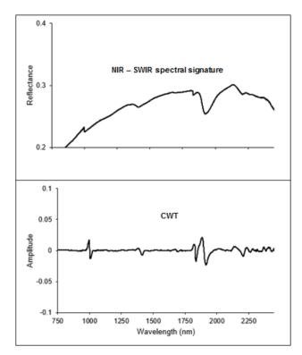
**Figure 2.** Example of the near-infrared (NIR) and shortwave-infrared (SWIR) spectrum and its continuous wavelet transform (CWT) for a soil sample that represents the highest SOC content over the study area. The wavelet is a Gaussian wavelet transform. Note the peak near to 1000 nm is an artifact due to detector offset.
