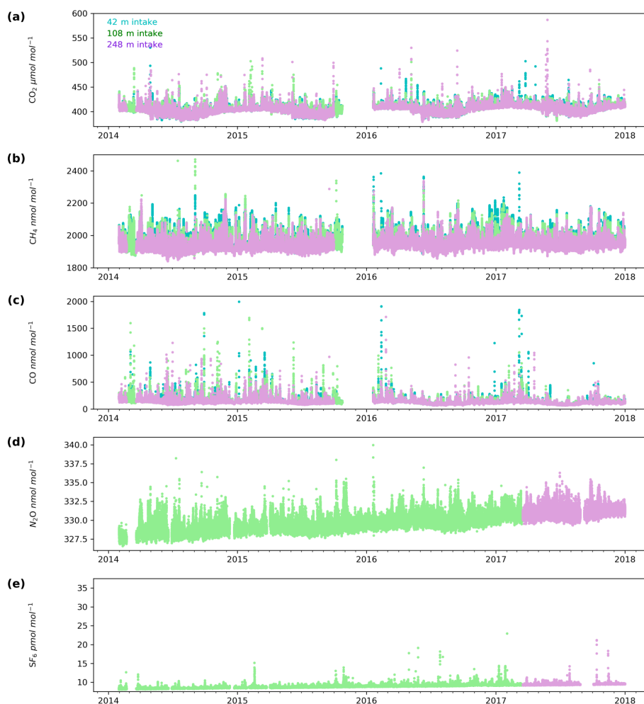
Figure 4. Minute-mean (a) \text{CO}_2 , (b) \text{CH}_4 and (c) \text{CO} and 10 min discrete (d) \text{N}_2\text{O} and (e) \text{SF}_6 observations at the Bilsdale site for the 42 m (blue), 108 m (green) and 248 m (purple) intake heights.
